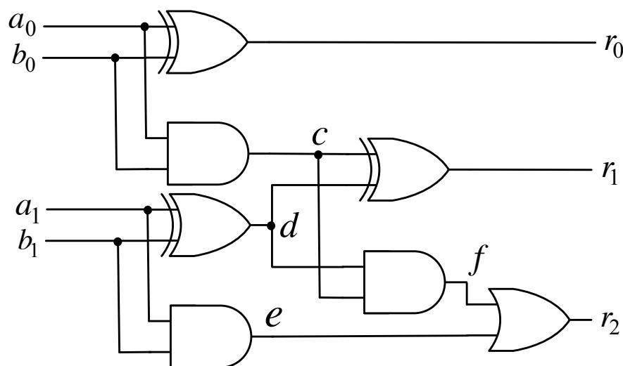
$$\left\{ \begin{array}{l} g_1 = r_0 - (a_0 + b_0 - 2a_0b_0) \\ g_2 = c - (a_0b_0) \\ g_3 = d - (a_1 + b_1 - 2a_1b_1) \\ g_4 = r_1 - (c + d - 2cd) \\ g_5 = f - (cd) \\ g_6 = e - (a_1b_1) \\ g_7 = r_2 - (e + f - ef) \end{array} \right.$$
